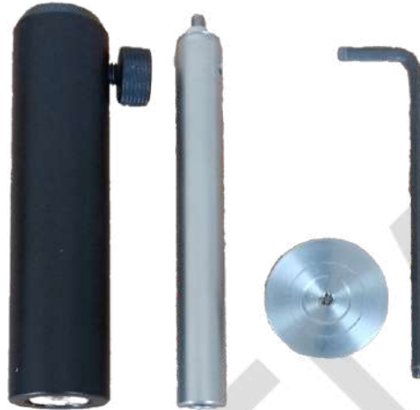
Figure 23. Optical post elements
