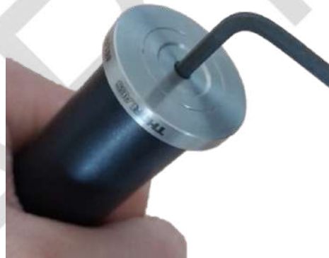
Figure 24. Base and post holder assembling
